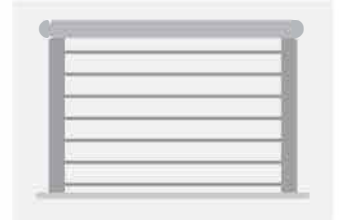
Steel Cable In-fill
